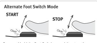
Press and hold the Foot Switch on and then turn the ON/OFF switch on. Lightly tap the foot switch to turn the e-Ball Winder ON and lightly tap again to turn it OFF. You can also operate your e-Ball Winder without the foot switch by turning it ON or OFF using the ON/OFF switch or speed control. However, our experience is that at full speed, the foot switch is a much more reliable way to stop tangles before they arrive at the yarn guide.
